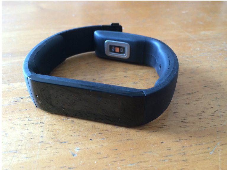
Figure 4.2: The Microsoft Band. The closest panel is a LED display which shows panels such as heart rate and GPS information. The metallic part in the back is the heart rate monitor.
